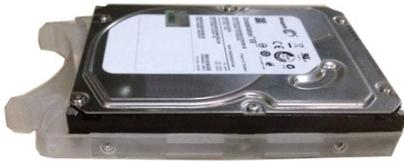
1. Line up the handle to the HDD side (without the interface)
