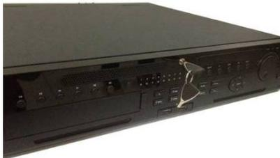
1. Turn the key into the hole in the front panel.
