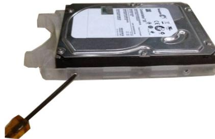
2. Use the screwdriver to fix the handle on the HDD.
